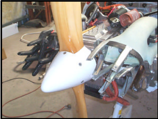
Clamp rubber while rubber is being glued.
