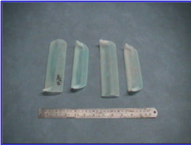
Reinforcing Aileron Hinge
