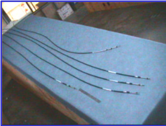
Cables: Aileronx2, Elevator, Rudder, Trim
